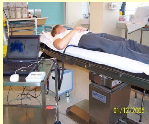
Fig. 2: Pressures recorded with the warming device superimposed on the operating table mattress using the maximum pressure settings of the device (60 mmHg)
