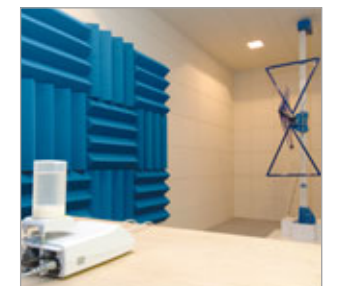
Electromagnetic wave measuring facility – Measuring electromagnetic waves radiated from products
